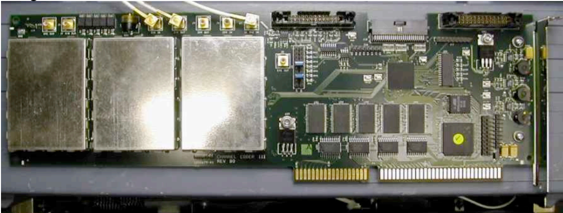
Figure 15 – Channel Coder Card Used for Distributed Transmission
