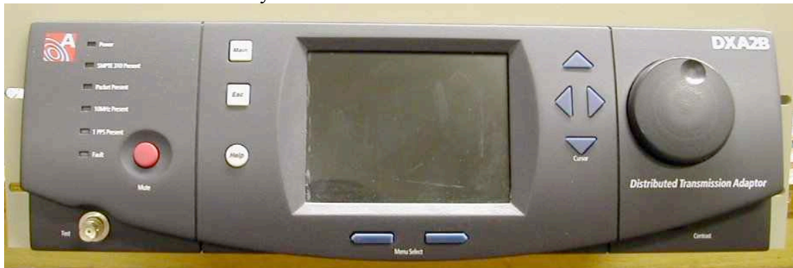
Figure 14 – A Distributed Transmission Adaptor (DTxA)
